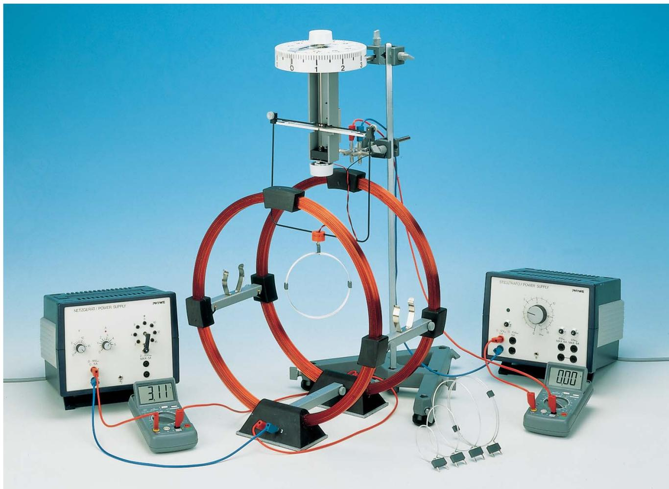
The zero-point of the torsion balance should be checked frequently, since rapid rotary movements can displace the connecting leads.
