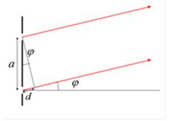
The two beams are practically parallel. The difference in length of the two beams is *d*. Constructive interference occurs when  $d = n\lambda$ , where *n* is an integer. From the right triangle (see the figure above) one sees that  $d = a \sin \varphi$ , where *a* is the distance between two neighbouring slits. It is called the constant of the grating and is usually specified by the manufacturer. Thus we have the following condition for the appearance of diffraction maxima:
