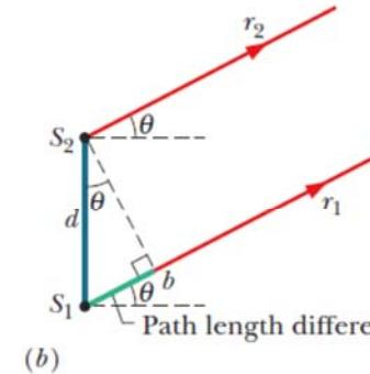
The  $\Delta L$  shifts one wave from the other, which determines the interference.
