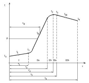
I - the temperature of the liquid is below room temperature. A moderate increase of the temperature could be observed due to the heat transferred from the ambient environment to the calorimeter. Record the data for about 5 minutes in this phase.
