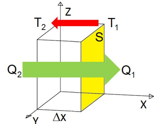
$$Q_1 - Q_2 = c\Delta m \Delta T = c\rho\Delta V \Delta T = c\rho S \Delta x \Delta T = -\Delta q S \Delta\tau$$
