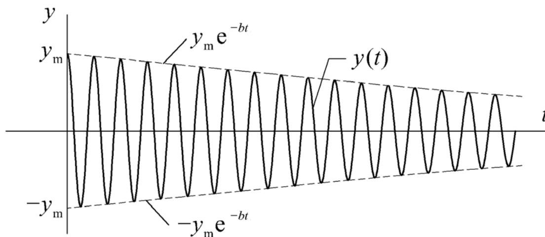
**characteristics:** damping ratio  $\beta = \frac{y_i}{y_{i+1}} = e^{bT}$
