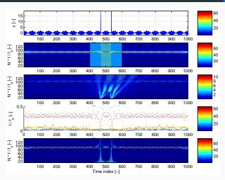
Harmonic signal with two pulses, STFT, WT, HHT and DZT spectrogram
